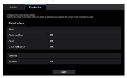
You can set event actions for SD schedule recording/FTP periodic image transmission/alarm detection. Once the settings are completed in each setup menu, click the [Next] button to proceed. The setup flow is as follows.
