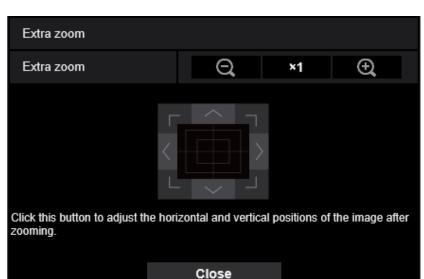
It is possible to adjust the angular field of view using the extra zoom function.
