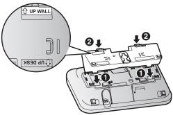
4 Mount the unit on a wall then slide down to secure in place.
