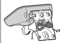
Mount the unit on a wall then slide down to secure in place.
