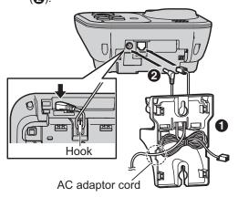
Insert the hooks on the wall mounting adaptor into holes (A) and (B) on the base unit.
