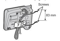
1 Drive the screws (not supplied) into the wall.
