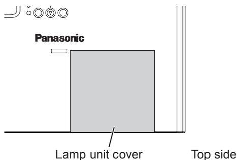
**3** Use a Phillips-head screwdriver to loosen the 2 lamp unit screws. Pull the used lamp unit gently from the projector.
