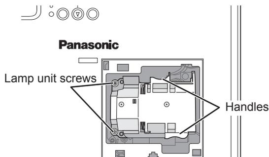
**4** Press in the lamp unit until it clicks and make sure the unit is installed securely. Tighten the 2 lamp unit screws securely with a Phillips-head screwdriver. During insertion, particularly press the (A) portion securely.
