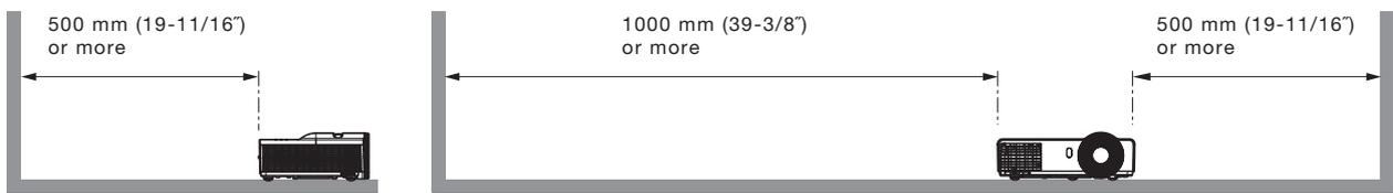
**Direction of air intake and exhaust**
