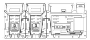
**3.** Connect the Ext jack on the host phone and the Ext in jack on the expansion module using one supplied cord.
