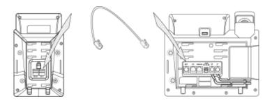
If you connect two expansion modules, connect the Ext out jack on the prior expansion module and the Ext in jack on the next expansion module using another supplied cord. Connecting two expansion modules on a single host phone is shown as below:
