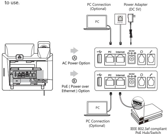
Note: The IP phone should be used with Yealink original power adapter (5V/2A) only. The use of the third-party power adapter may cause the damage to the phone. If you are connecting a PC to your phone, we recommend that you use the Ethernet cable provided by Yealink.
