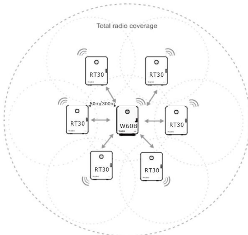
The maximum number of handsets that can be registered to your base station is not affected by the repeater. The repeater can be used to extend the coverage range in all directions, allowing several floors to be covered.
