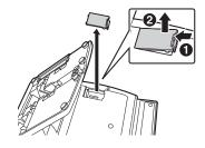
Plug the flat cable into the connector (1), then bend the cable slightly as shown (2).
