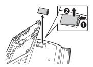
3. Plug the flat cable into the connector (♠), then bend the cable slightly as shown (♠).
