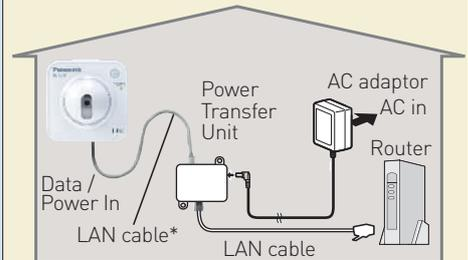
\*Use a LAN cable that is no more than 30 m (98 feet 5 inches) long to connect the camera and the power transfer unit.
